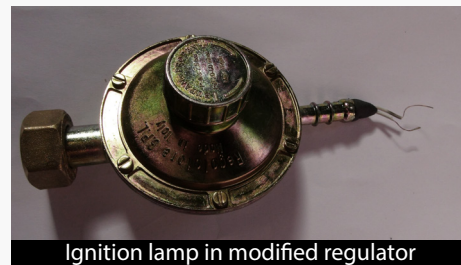
Ignition lamp in modified regulator
